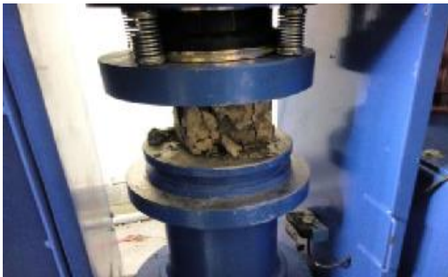
Figure 1: Failure of concrete block
