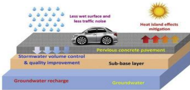
Fig. Pervious Concrete in roads
