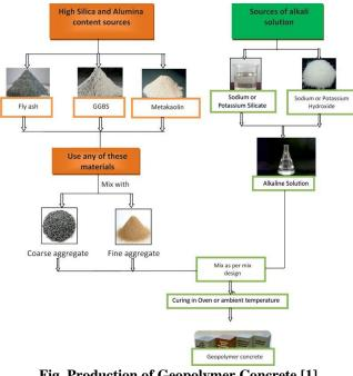
Fig. Production of Geopolymer Concrete [1]
