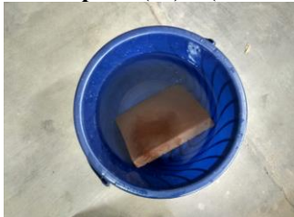
Figure 15. Water Absorption Test
