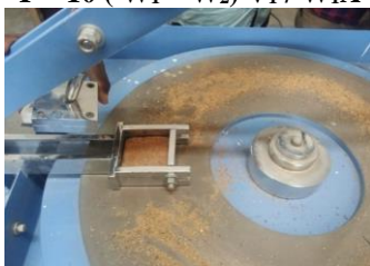
Figure 16. Tile Abrasion Test
