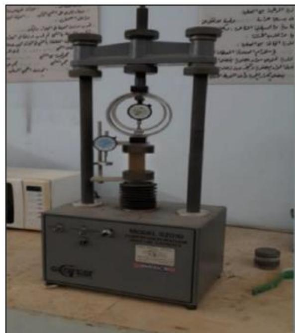
Figure (2): Unconfined compression test used to determine the unconfined compression strength of samples.
